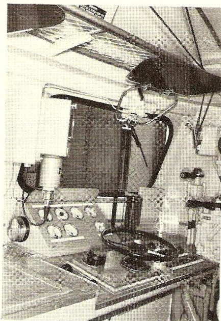
Driving controls at right-hand side of cab
