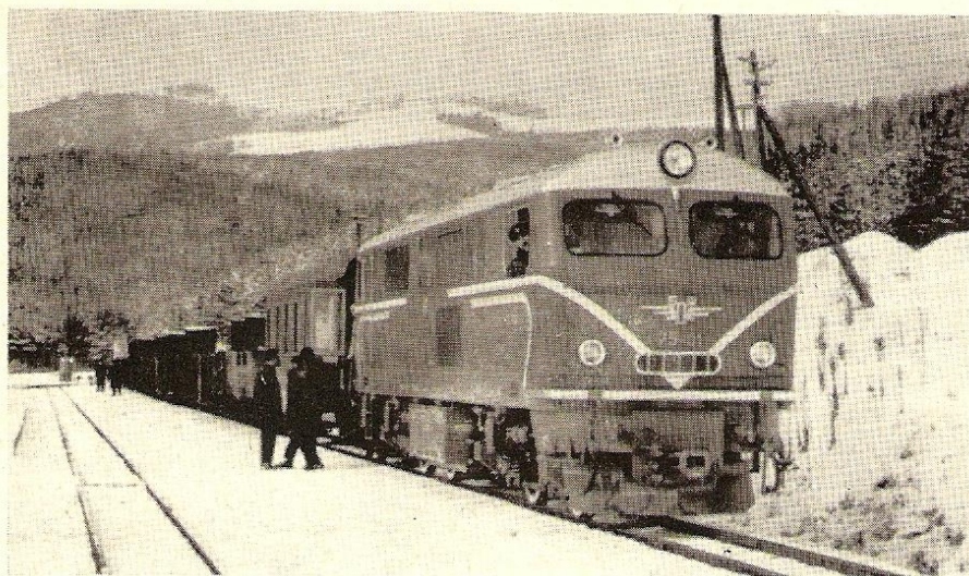
Load test in progress with the first Henschel B-B series 75-01 diesel-hydraulic
