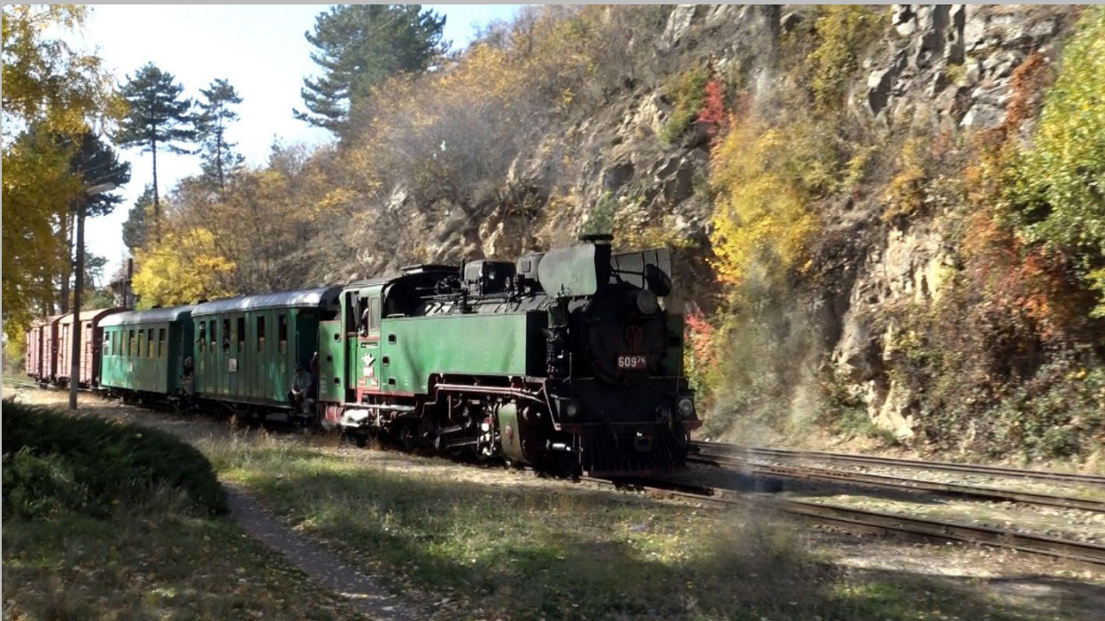
609. 76 is the narrow gauge (760mm) 2-10-2T built by Chrzanow in Poland, works No. 1929 of 1935 The superscript 76 indicates the gauge in cms.
