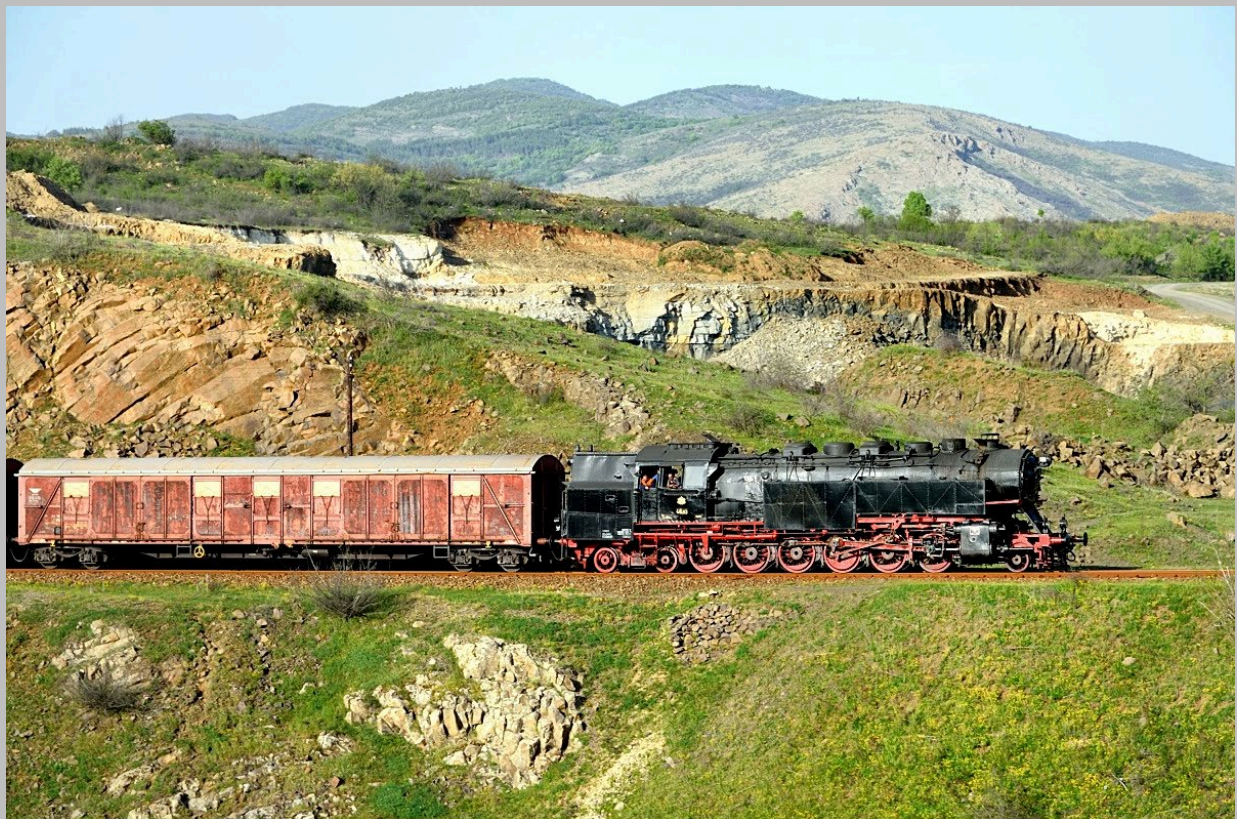
This massive 2-12-4T, built in Poland in 1931 by Cegielski of Poznan, was until recently under repair, but it was outshopped to work children's Christmas Specials in December 2024. Photo courtesy Daniel Simon.
